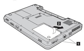
6 Pull the tab in the direction shown by arrow 3.
